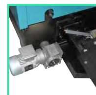
Gearmotor of automatic ash removal system
